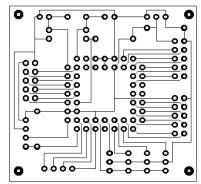
I will place all my printouts and documentation on the SRS BBS. (206) 362-5267. The file will also contain the PADS circuit if you want to play with it. The print files can be used to create a board using the heat transfer method.
