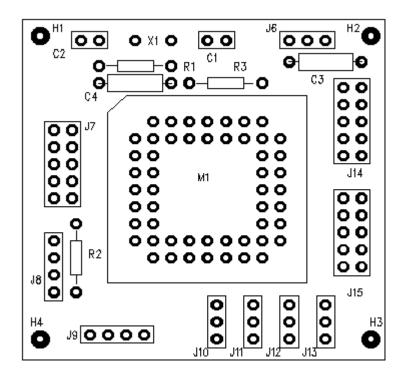
With those goals in mind I also wanted to have power supply pins on each header, four servo ports, separate serial and SPI ports, and a small prototyping area. Later I decided against the prototyping area because it would increase board size, and proto boards can be purchased cheaply from Radio Shack and Digi Key etc.
