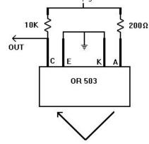
The software could read the analog value and determine the difference between a dark line and white paper. allowing the robot to 'see' a black line. This sensor can also be used for many other purposes like an obstacle detector, maybe a hand sensor etc. The sensors small size allow to fit just about any ware.
