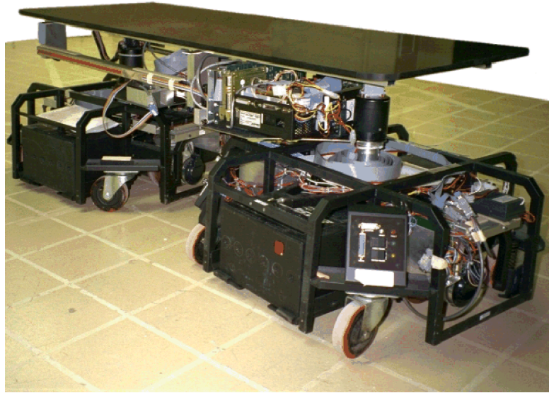
Figure 4.3: The CLAPPER is a unique 4-DOF mobile robot developed at the University of Michigan. The CLAPPER can measure and correct non-systematic dead-reckoning errors during motion.
