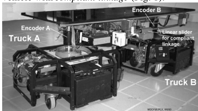
Figure 1: The University of Michigan's experimental dual differential drive vehicle with compliant linkage.
