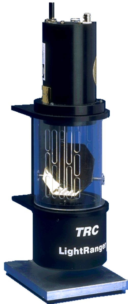
Figure 4.28: The TRC Light Direction and Ranging System incorporates a two-axis scanner to provide full-volume coverage sweeping 360° in azimuth and 45° in elevation. (Courtesy of Transitions Research Corp.)
