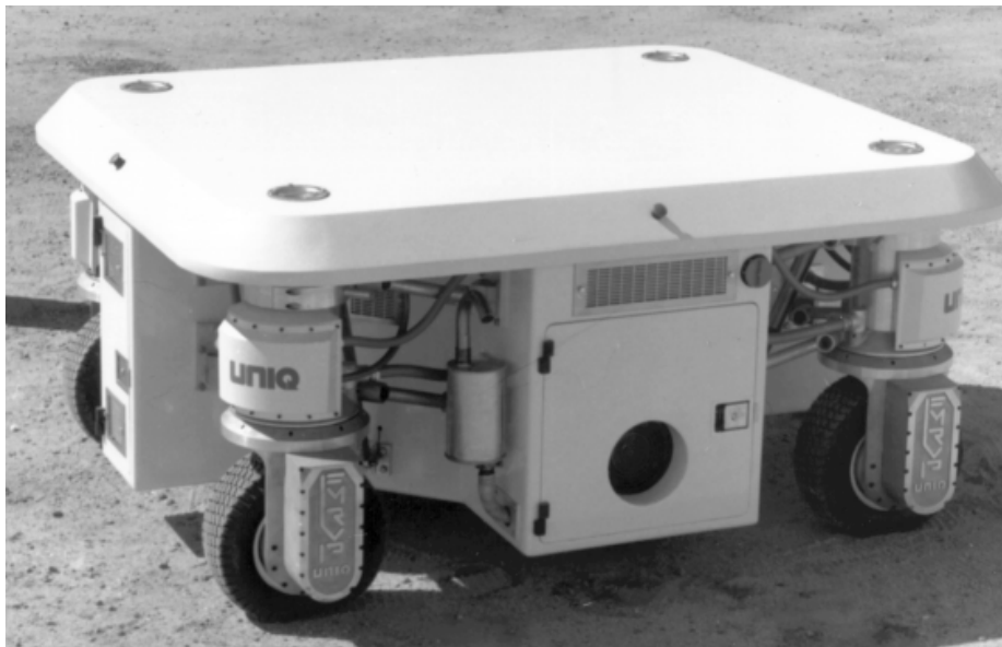
Figure 1.14: An 8-DOF platform with four wheels individually driven and steered. This platform was designed and built by Unique Mobility, Inc. (Courtesy of [UNIQUE].)
