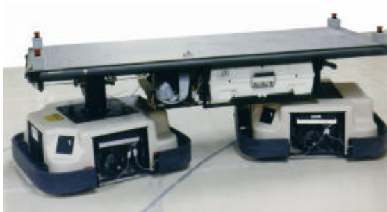
Figure 1: The OmniMate is based on two TRC LabMate "trucks" connected by a compliant linkage. This design provides a free 180x90 cm (72x36-in) loading deck for up to 114 Kg (250 lbs) of payload.
