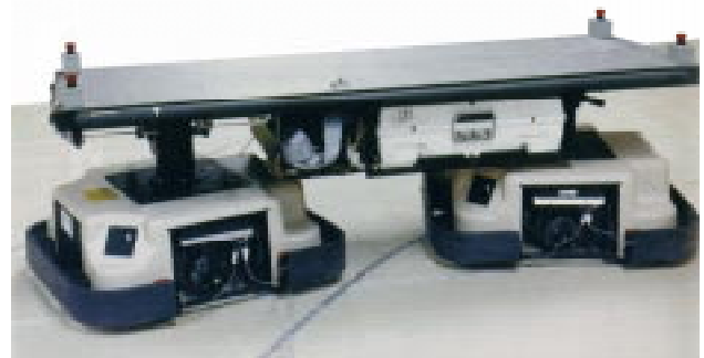
Figure 1: The OmniMate is based on two TRC LabMate "trucks," connected by a compliant linkage.
