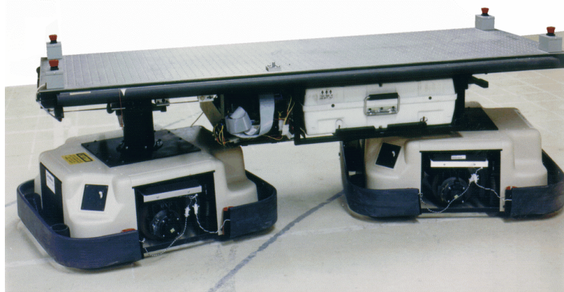
Figure 3: The OmniMate is a commercially available fully omnidirectional platform. The two linked “trucks” mutually correct their odometry errors.
