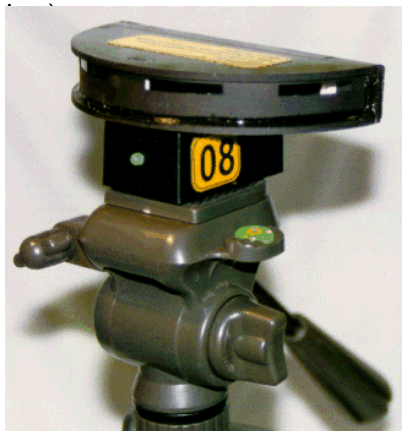
Figure 8: Stationary NOADs are located at known positions; at least two NOADs are networked and connected to a PC. (Courtesy of MTI Research, Inc.)
