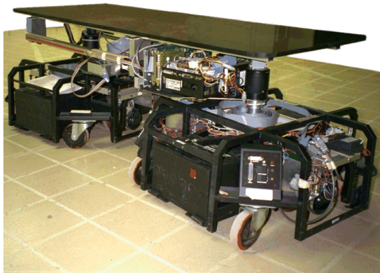
Figure 1: The University of Michigan's experimental dual differential drive vehicle with compliant linkage.
