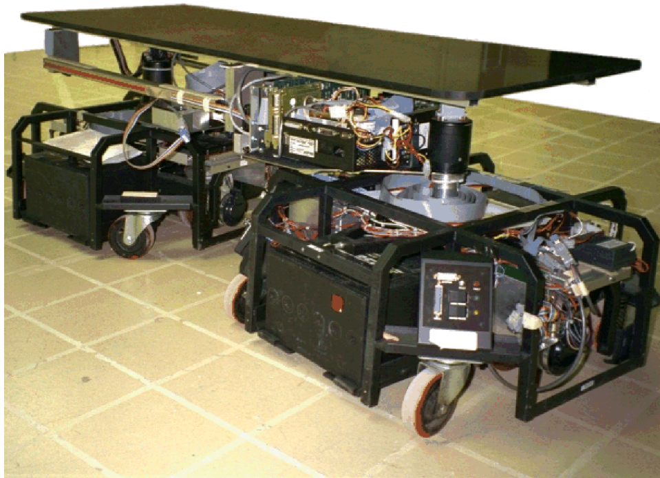
(32) Figure 11: The experimental dual differential drive vehicle, built and tested at the University of Michigan
