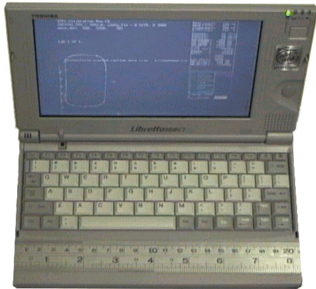
Figure 2: The Toshiba Libretto 100 CT is a 2.2-pound miniature notebook computer that serves as the main onboard PC. It features a 166 MHz Pentium processor, 32 MB RAM, and a 2.1 GB harddisk.
